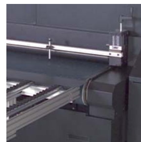
Separate media loading zone and print zone for accurate media feed.
