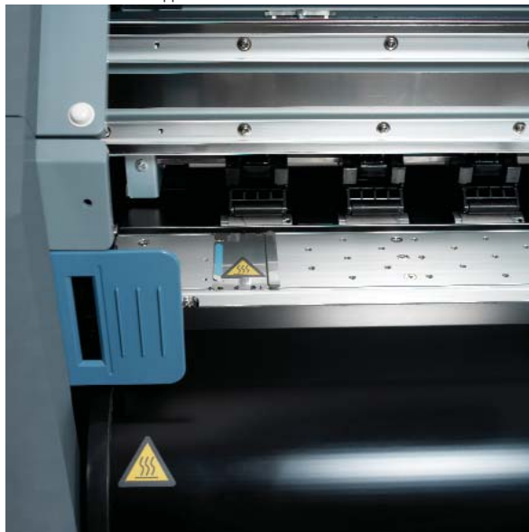
Edge guard & integrated heater
